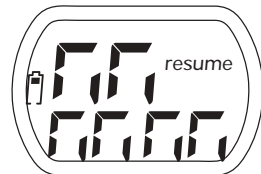
test pattern 2 (alternate segments activated)
