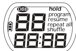
test pattern 2 (alternate segments activated)
